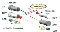
Product with FiberAlert enabled —Remote Site stops transmitting Local Link LED is OFF indicating a break in the fiber loop
